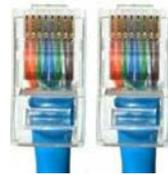
All the Cat-5 cable you can get your hands on at retail has solid conductors. This type of cable will fail on shipboard due to vibration. You really should go on the internet and find stranded Cat-5 cable and the special RJ-45 connectors made for it.
